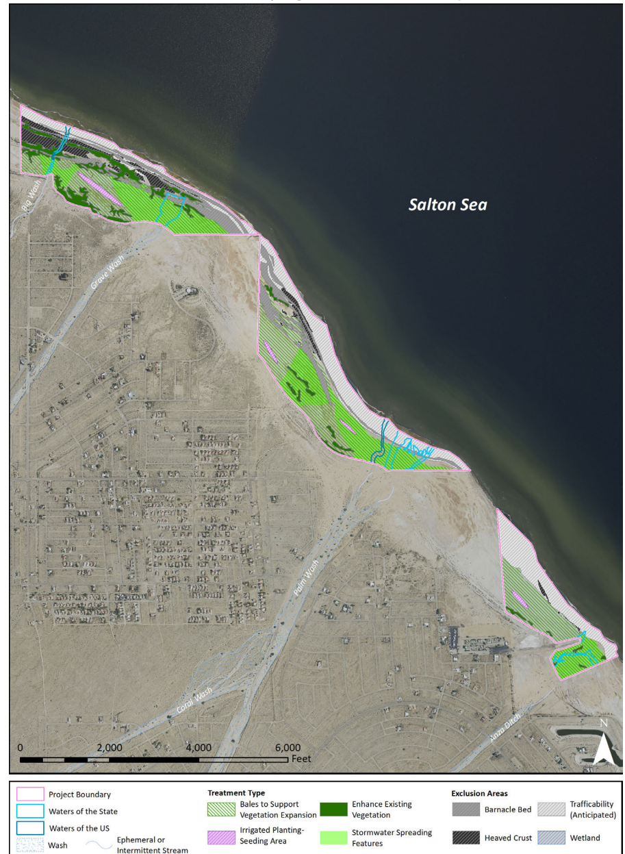
Figure 6. Initial layout of vegetation enhancement project at the Clubhouse site (see Figure 3 for general site location). The colored areas within the site are Reclamation-administered land, with the colors indicating the extent of vegetation cover and whether the land is below the ordinary high-water mark or an aquatic habitat.
