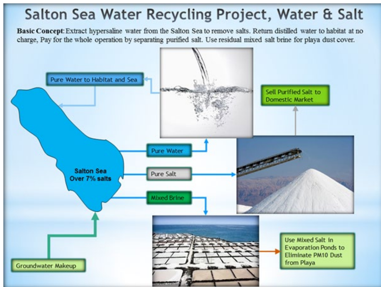
Figure 5-29. Illustration of Concept 7: Salton Sea Water Recycling, Graphic Provided by Sephton Water Technology.
